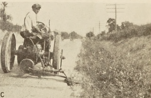
A, THE HORSE-DRAWN FARM MOWER IS STILL THE MOST COMMONLY USED MOWING UNIT ON ROADSIDES. B, MOWER BEING PULLED BY A LIGHT TRUCK. C, TRACTOR WITH POWER TAKE-OFF FOR OPERATING MOWER.
